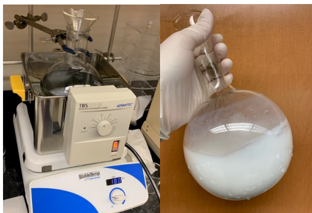
Figure 2: The Ti(IV) solution is placed in a water bath at 40 °C for 4 days (left). The reaction results in the white, gelatinous TiO 2 being formed (right).
