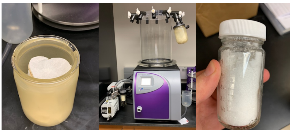
Figure 5: The frozen tubes were covered in a filter and placed into a jar (left), which is attached to a freeze-dry apparatus (center). After 24 hours at 200 mTorr, the TiO 2 nanocrystals have been obtained in powdered form (right).
